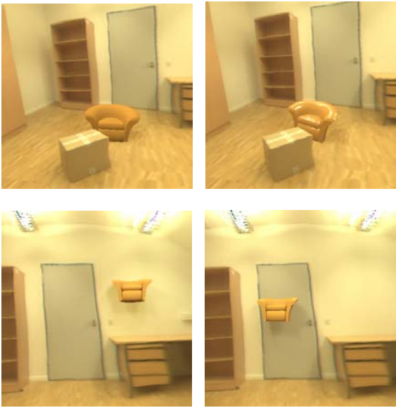
Figure 6. A virtual armchair, illuminated by 32 important light patches, is inserted. The upper right image shows the armchair with a floating-point reflection map. The lower row shows the virtual object and the light sources. The chair can be moved at 3..20 fps (32..2 important lights)
