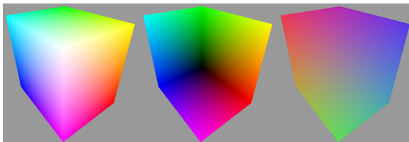
Figure 3: Color-coded textures to generate rays: starting positions (left), end positions (middle) and resulting normalized vectors (right).
