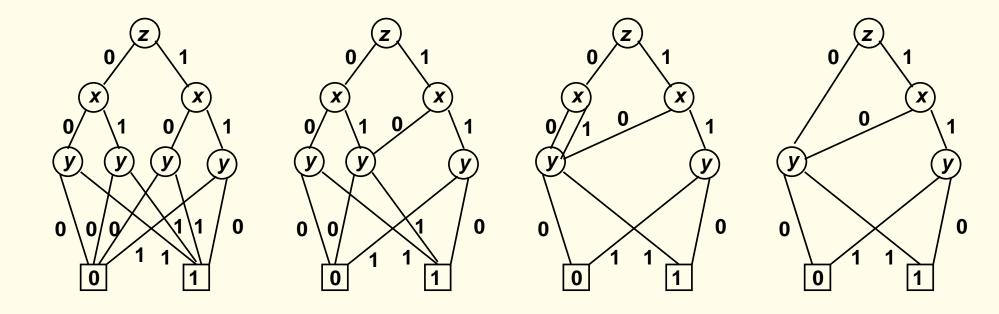
The algorithm reduce traverses an OBDD B layer by layer in a bottom-up fashion, beginning with the terminal nodes.
