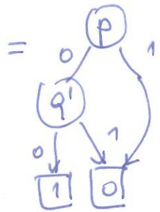
$\text{exists}(q', B_{f'}) = \text{apply}(\vee, \text{restrict}(0, q', B_{f'}), \text{restrict}(1, q', B_{f'}))$
