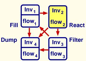
**Mode 2: React** Temparature is high. Substances 1 and 2 react. The reaction consumes equal quantities of substances 1 and 2 and produces substance 3.
