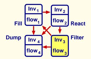
If proportion not kept: system jumps into mode 4 (**Dump**); Otherwise, if the concentration of substance 3 is below some minimal level min the system jumps into mode 1 (**Fill**).
