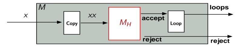
Case 1: *M* started with G(M) halts: Then  $G(M)G(M) \notin HALT$  Contradiction! Case 2: *M* started with G(M) does not halt: Then  $G(M)G(M) \in HALT$  Contradiction! **Theorem.**  $K = \{G(M) \mid M \text{ halts for input } G(M)\}$  is acceptable but undecidable.
