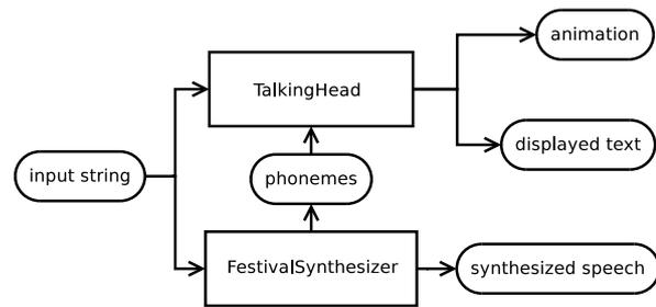
Figure 4: Components and interaction of the robot face.
