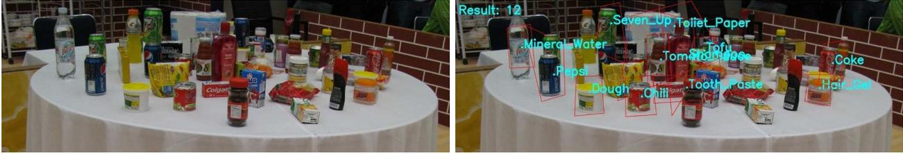
Figure 4. The input image for object recognition as acquired by our robot during the Technical Challenge of the RoboCup (left). Object recognition results with 12 correctly identified object instances (right).
