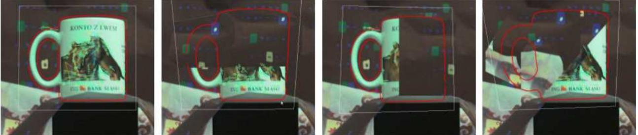
Figure 3. Example images for detection of partially occluded objects. From left to right: the unoccluded object is recognized with 98 matched features and 38% confidence. The occluded object have less features, but are still recognized correctly: 49 with 33 %, 17 with 17 %, and 34 with 34 %.
