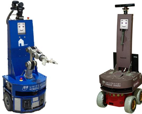
**Fig. 1.** Setup of our 2 robots. The current setup of Lisa is shown on the left. With this setup, Lisa is participating in the RoboCup since 2014 and is now our main robot. An older version of Lisa is shown on the right. This setup is the auxiliary robot of our team.
