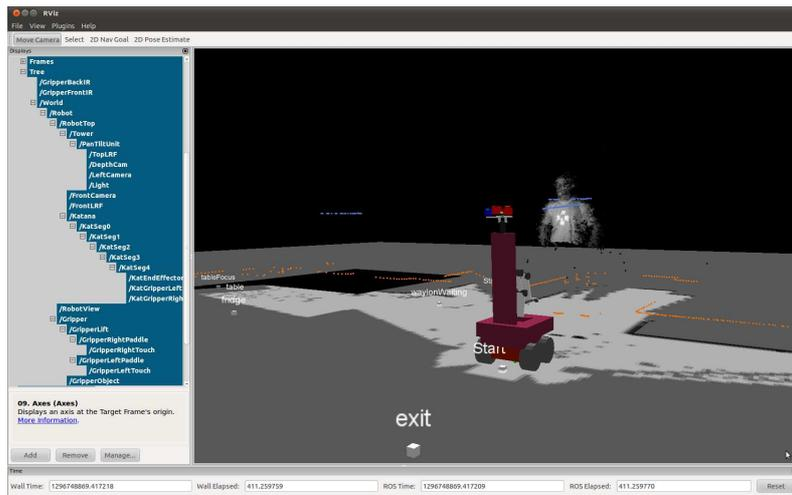
**Fig. 3.** The rviz visualization tool showing various visualizations of sensor data. The application can be used for real-time surveillance of the robot as well as for playing back recorded sensor log files of R16 and ROS. In the @Home league, this is mainly used by the developers for testing and evaluation.
