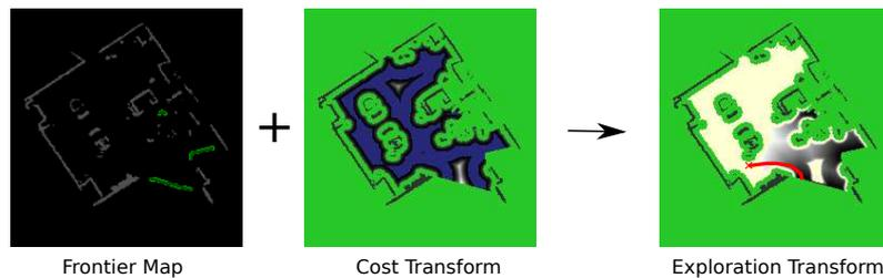
**Fig. 5.** Illustration of the exploration transform algorithm described in [WP07]. The left image shows the extracted frontiers. The blue area in the middle image contains accessible areas. The red line in the right image represents the path of the robot. The dark values indicate a short distance to the next safe frontier, white cells indicate a long way.
