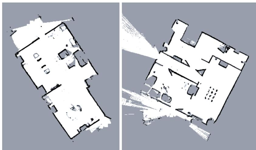
**Fig. 4.** Real-time maps of the RoboCup 2008 (left) and 2009 (right) @Home arena.
