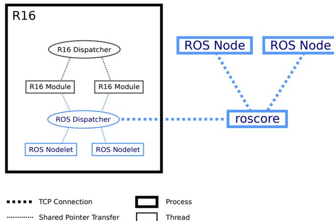
**Fig. 2.** Schematic description of the communication between R16 and ROS.
