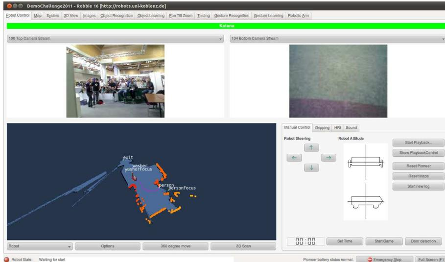
Figure 4: GUI during the Demo Challenge competition of the RoboCup@Home in Magdeburg (2011): top camera view (top left), bottom camera view (top right), 3D-view with scene graph of robot, map and navigation path, points of interest and laser data (bottom left). Control elements are located on the bottom right that allow to manually control the robot, gripping or human-robot interaction related tasks.
