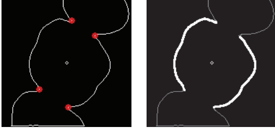
Fig. 3. Left: split points of the main contour. Right: contour segments after splitting.
