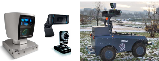
Figure 1: Deployed sensors and robot: A 3D laser range finder and two different commercially available cameras are used to perceive the environment. Sensors are mounted on top of a 500 kg outdoor robot.
