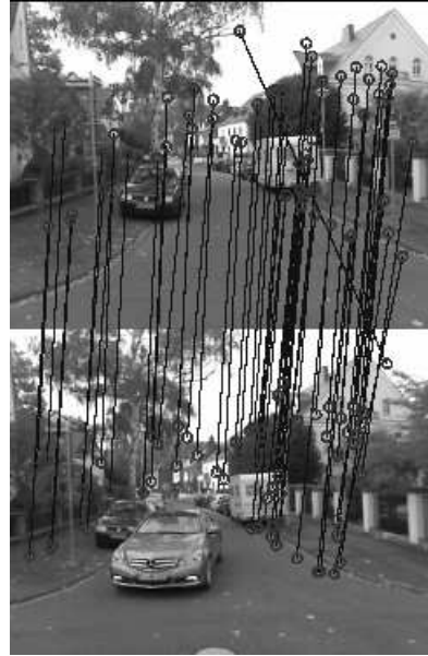
(b) Results of the image feature matching. Circles are illustrating SURF features and lines mark matched correspondences of the features.
