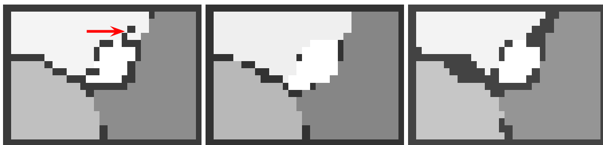
Figure 9: Section of a thermographic image. Vincent- (left), p_m = 51\% (middle) and p_m = 67\% (right). Black lines mark detected watersheds. The arrow marks the mentioned problem of the original algorithm.
