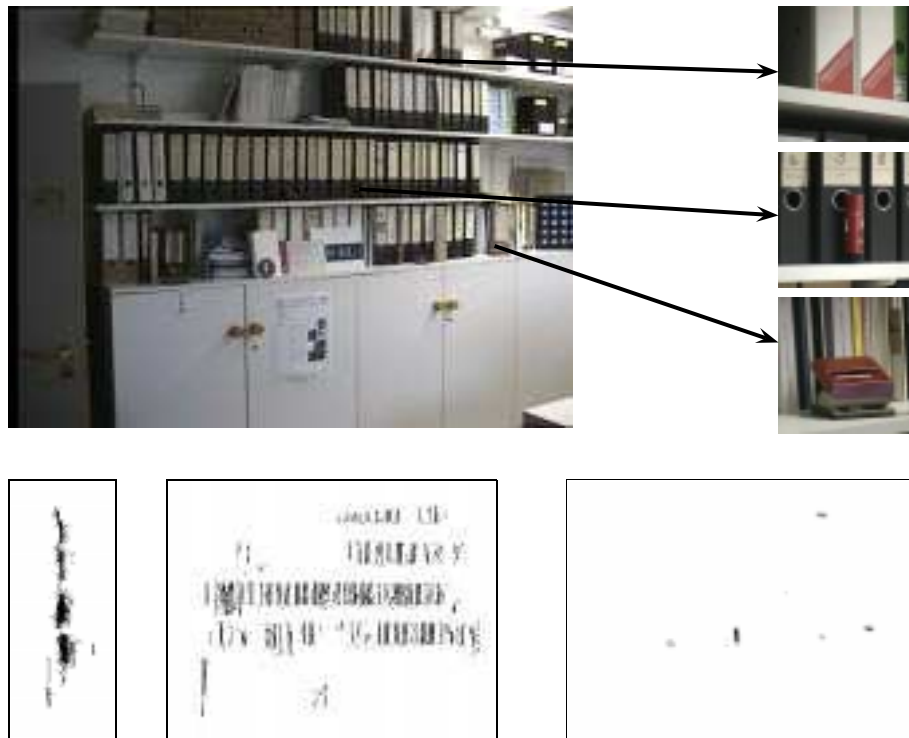
Figure 3.19. Office scene (top left), close up views used for hypotheses (top right), two projections of 3D points (bottom left), color backprojection for red punch (bottom right). The red punch searched for is shown in the close-up views on the top right.
