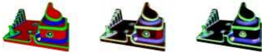
Figure 3.11. Example of range image segmentation. Result of segmentation rendered with different colors corresponding to regions of different curvature characteristics (left). The other two images additionally show the minimal and maximal curvature coded by the brightness of the color.
