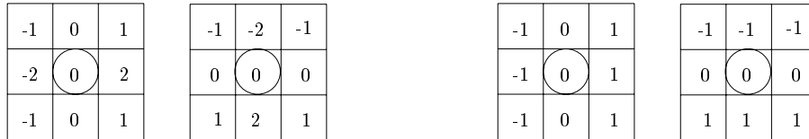
Figure 3.3. Masks for Sobel (left) and Prewitt (right) operator. Masks on the left: f_x , masks on the right: f_y . Note that these masks may be flipped with respect to other literature since we choose the origin of the coordinate system on the left top.
