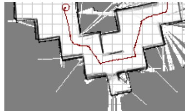
(c) Map generated from data of an adjusted LRF.
