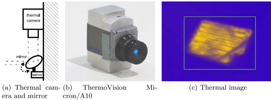
Fig. 2. Thermal camera mounting (a) and image of the thermal camera (b).
