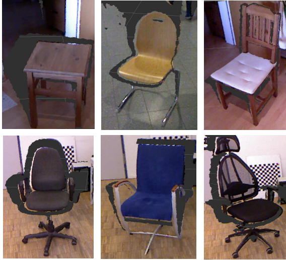
Figure 1: Example furniture objects corresponding to the different fine-grained affordances detected by the presented approach. Top row: a stool representing the sitting without backrest affordance and two chairs representing the sitting with backrest affordance. Bottom row: three chairs representing the sitting with backrest and sitting with armrest affordances. Additionally, the rightmost chair also supports the sitting with headrest affordance.
