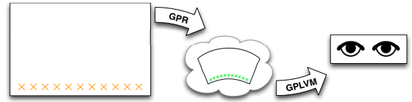
Fig. 2: System Overview of the gaze tracker. First, a small sample set of eye-patches and the corresponding gaze points in screen coordinates are captured. Second, the Gaussian process latent variable model [6] is used to compute a lower dimensional gaze manifold from eye-patches. Third, Gaussian process regression is used to establish a mapping from screen coordinates to eye-patches.
